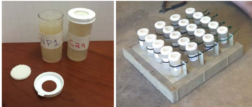
Figure 2. The left panel shows the tubes filled with agar. The left tube is unassembled showing the tube filled with agar, porous glass disk, and cap. The right tube is fully assembled. The right panel shows the tubes being tied into the tray.
